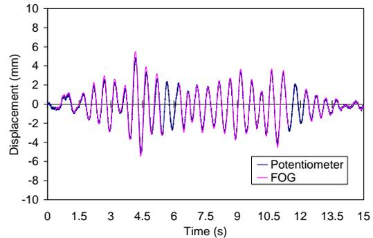
(c) Relative displacement at first floor
