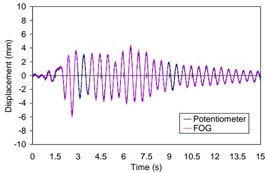
(c) Relative displacement at first floor
