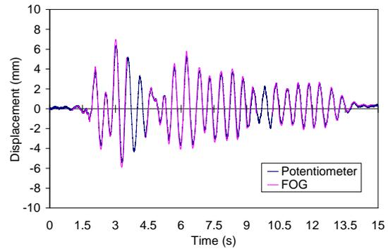
(c) Relative displacement at first floor
