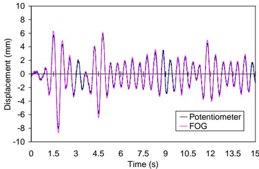
(c) Relative displacement at first floor
